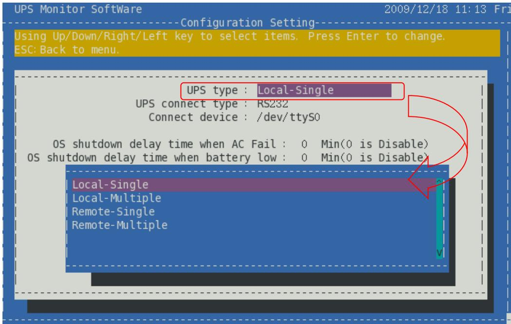
Use the directional key to select UPS type. You can set monitoring mode which is local or remote monitoring, and machine mode is single or multiple. Selectable items as below:
