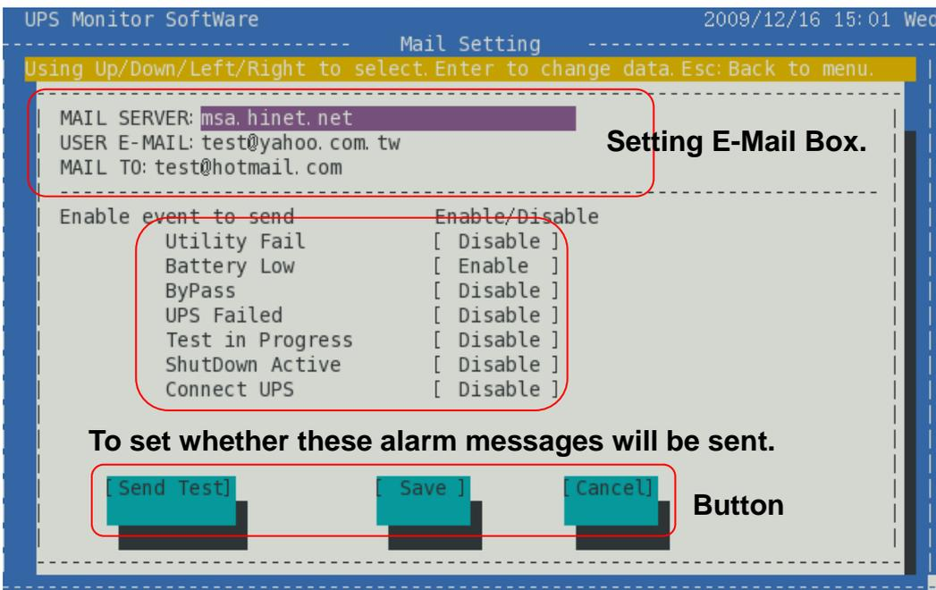
In event of power failure or abnormality, the “E-Mail” function automatically informs user via email. User can select alarm messages to meet the requirement. Ensure the E-Mail account is correct and the alarm message is enabled. Click [Save] to save all settings.
