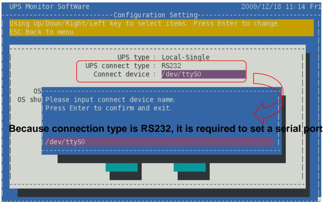
Because connection type is RS232, it is required to set a serial port
