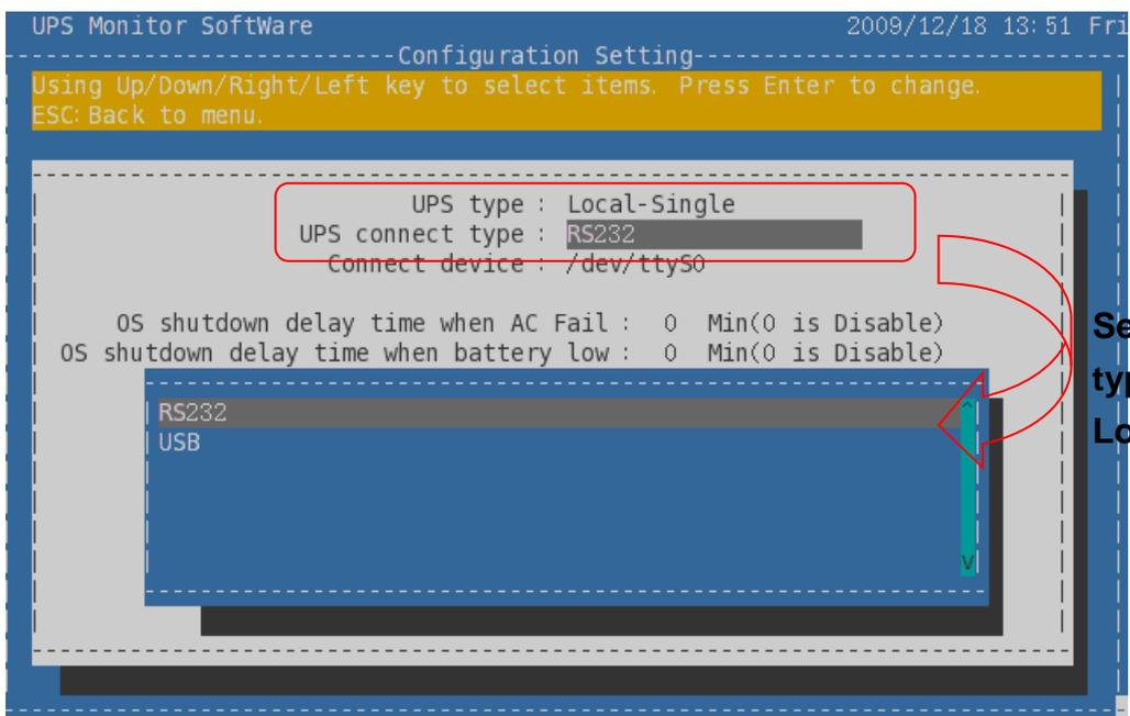
**Setting UPS connect type is required for Local monitor.**
