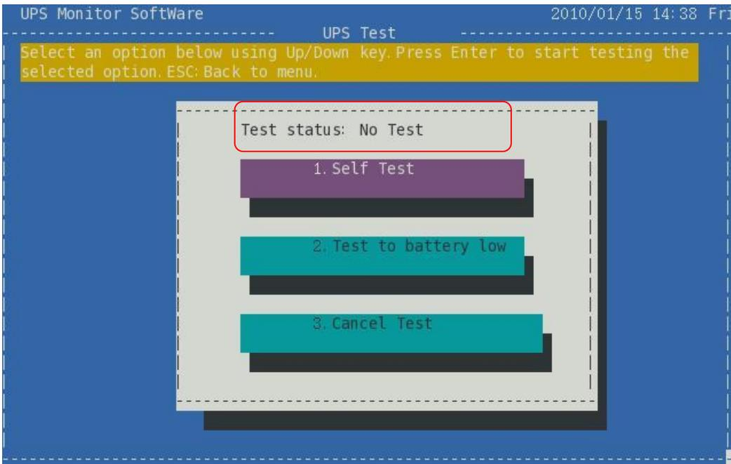
UPS Test includes: Self Test, Test to battery low and Cancel Test. Use the directional key to select the type of test. Then press the Enter key to execute or cancel test command. The screen display current test status and real time monitoring information. "Test in progress" indicates the machine is executing test command. "No Test" indicates that no test command is executed.
