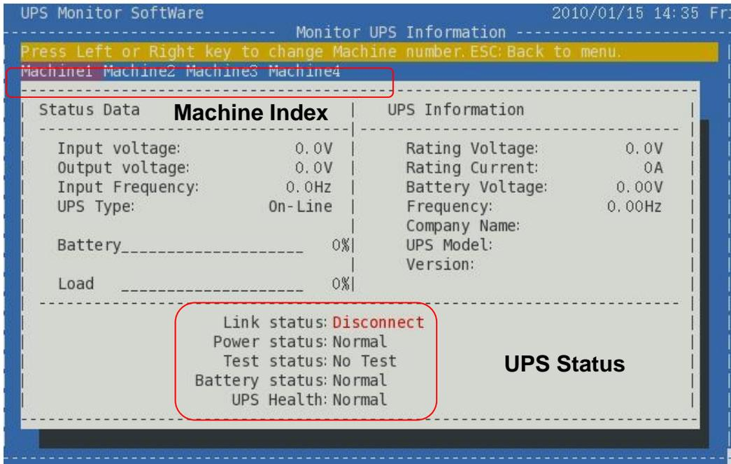
LinuxEmily is capable of monitoring and display information of four UPS. Use the directional key to switch between machine index. The information and status of UPS is updated immediately according to the selected machine index. Besides UPS real time information, it also displays Link status (communication), Power status (utility), Test status, Battery status and UPS condition.
