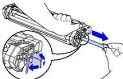
Holding the toner cartridge, pull the sealing tape straight to remove it from the cartridge. Be careful not to cut the tape. If this happens, you cannot use the toner cartridge.
